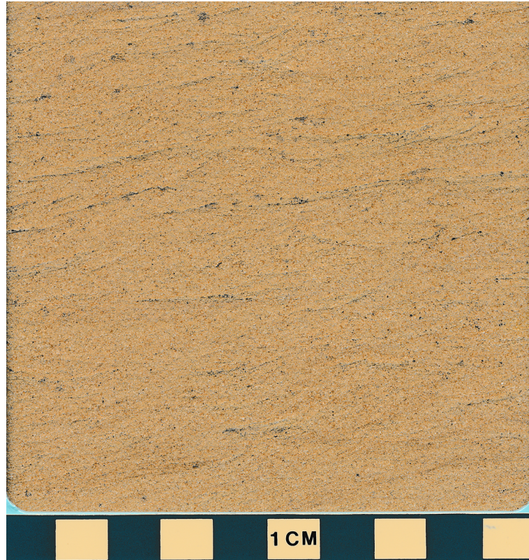
Fig. 5. Typical drab-colored sandstone (very fine-grained) from the el-Mahamid quarry.
